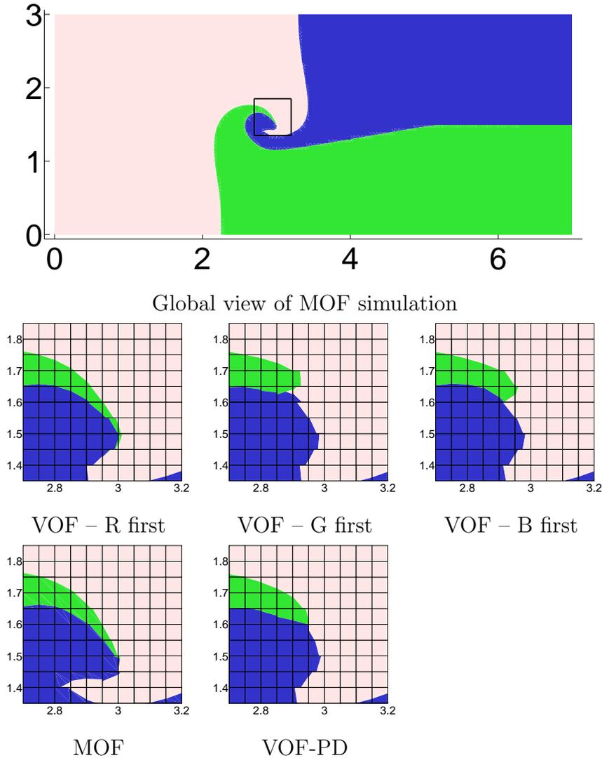
Fig. 6. Materials of triple point problem simulation, time  $T = 2.5$ . Eulerian runs (as Lagrangian step and remap to the initial orthogonal mesh) using different methods for material reconstruction are shown: global view on the entire computational domain for MOF method, and zooms to the three material junction for Young’s VOF method (with different material orderings), MOF, and Power Diagram based methods are shown.
