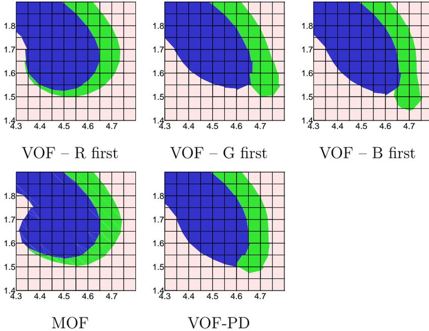
Fig. 7. Materials of triple point problem simulation, time  $T = 5.0$ . Eulerian runs (as Lagrangian step and remap to the initial orthogonal mesh) using different methods for material reconstruction are shown: global view on the entire computational domain for MOF method, and zooms to the three material junction for Young’s VOF method (with different material orderings), MOF, and Power Diagram based methods are shown.
