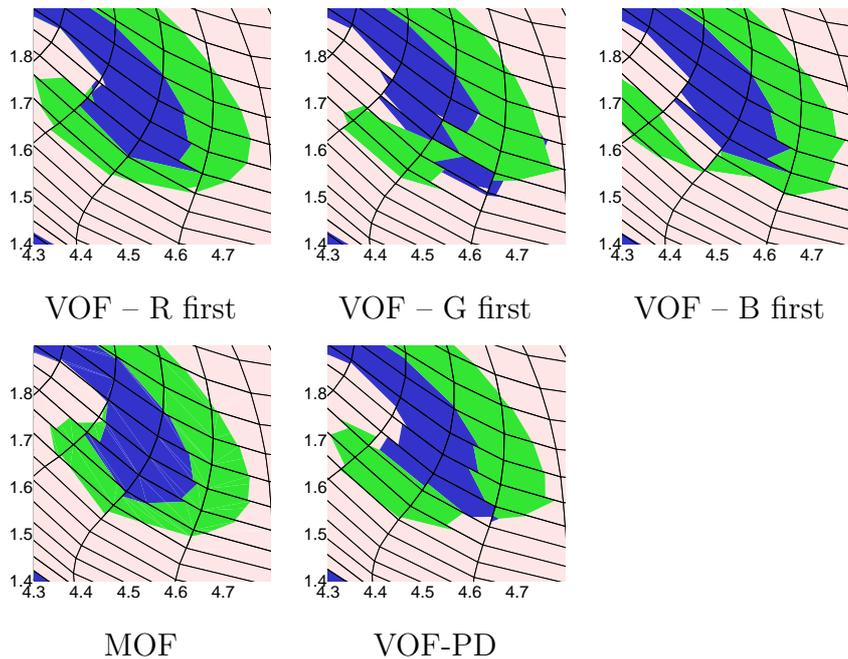
Fig. 10. Materials of triple point problem simulation, time  $T = 5.0$ . ALE runs (as Lagrangian step and remap to the Winslow smoothed mesh after every 20 Lagrangian steps) using different methods for material reconstruction are shown: global view on the entire computational domain for MOF method, and zooms to the three material junction for Young’s VOF method (with different material orderings), MOF, and Power Diagram based methods are shown.
