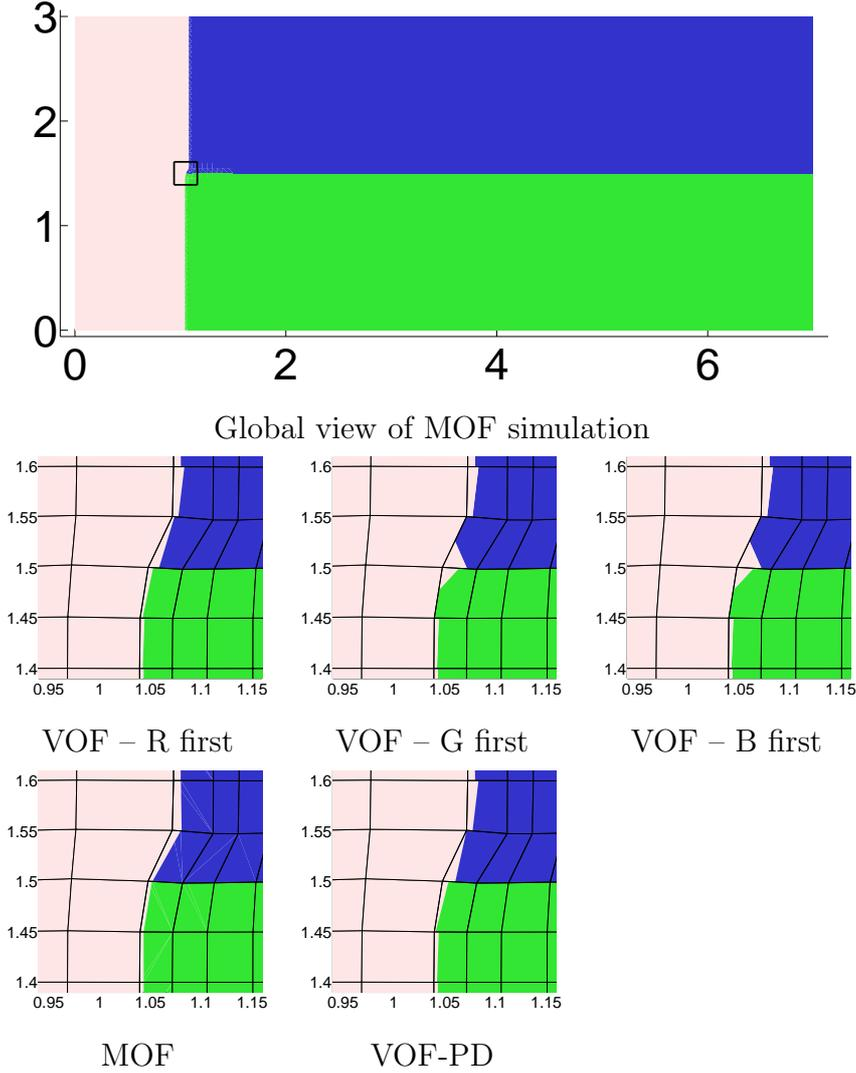
Fig. 8. Materials of triple point problem simulation, time  $T = 0.1$ . ALE runs (as Lagrangian step and remap to the Winslow smoothed mesh after every 20 Lagrangian steps) using different methods for material reconstruction are shown: global view on the entire computational domain for MOF method, and zooms to the three material junction for Young’s VOF method (with different material orderings), MOF, and Power Diagram based methods are shown.
