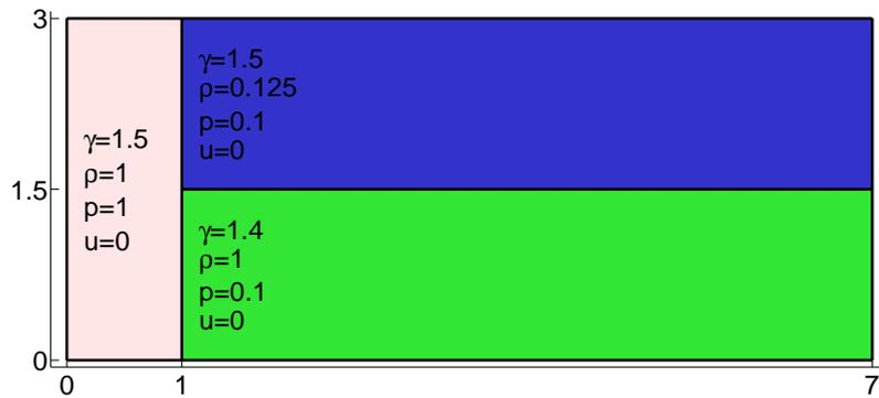
Fig. 4. Initial conditions for static triple point problem. Materials are shown in different colors, and values of ratio of specific heats  $\gamma$ , density  $\rho$ , pressure  $p$ , and velocity  $u$  are listed.
