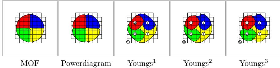
Fig. 2. Four material disk at time  $T = 0.5$  translated from the initial position  $(0.2, 0.2)$  with 30 time steps at a velocity of  $(1, 1)$  on  $32 \times 32$  mesh of the  $[0, 1]^2$  domain. Material reconstruction done by several methods – MOF, VOF with power diagrams, and Youngs’ VOF. The material orderings for Youngs’ are indicated in the figure.
