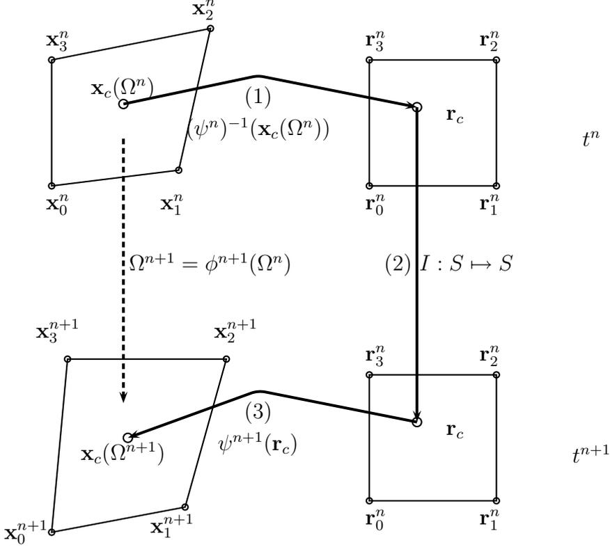
Fig. A.1. Steps in the constant parametric coordinate method. (1) The logical coordinates of the centroid at time  $t^n$  are calculated. (2) It is assumed the centroid has the same logical coordinates at time  $t^{n+1}$ . (3) The logical coordinates are mapped to physical coordinates to give the location. This gives a second order accurate approximation to the centroid of the evolved region  $\Omega^{n+1} = \phi^{n+1}(\Omega^n)$ .
