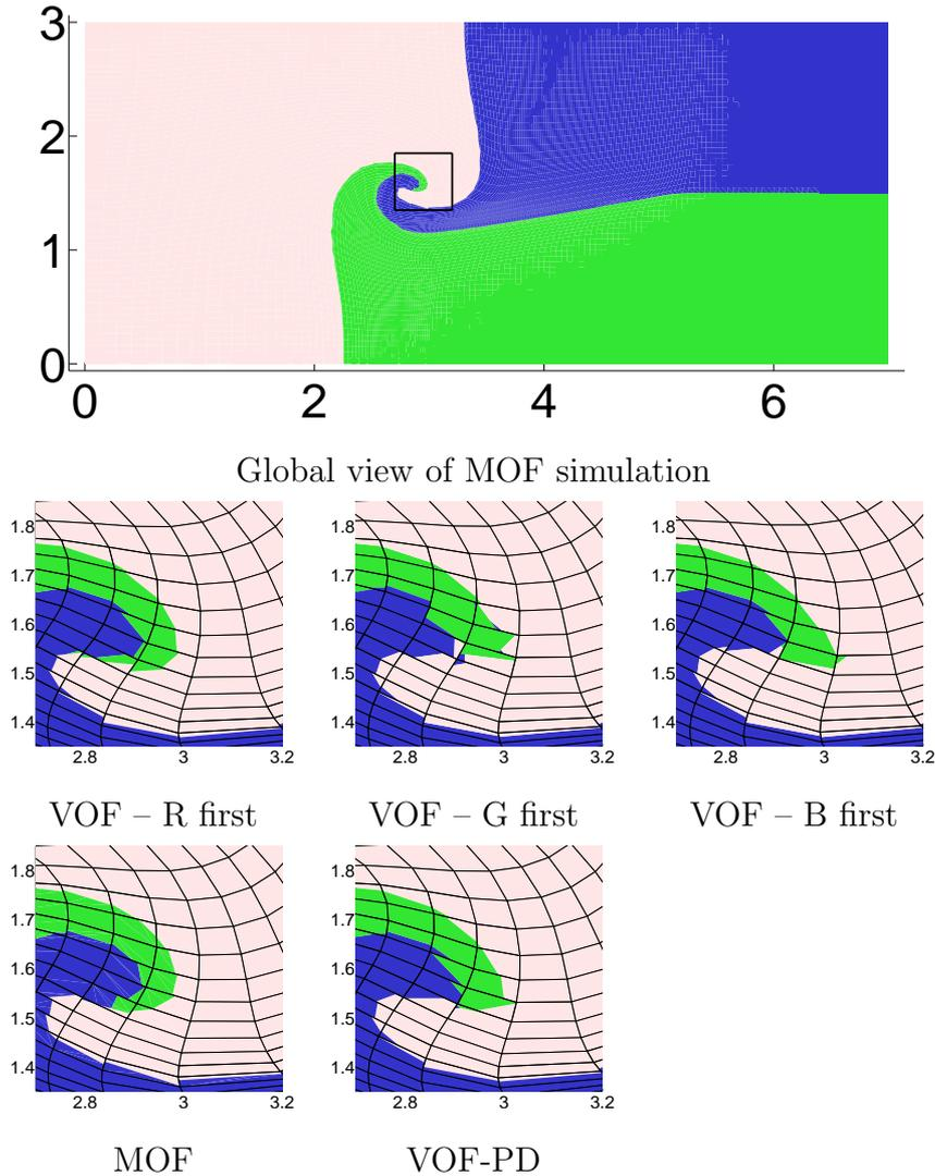
Fig. 9. Materials of triple point problem simulation, time  $T = 2.5$ . ALE runs (as Lagrangian step and remap to the Winslow smoothed mesh after every 20 Lagrangian steps) using different methods for material reconstruction are shown: global view on the entire computational domain for MOF method, and zooms to the three material junction for Young’s VOF method (with different material orderings), MOF, and Power Diagram based methods are shown.
