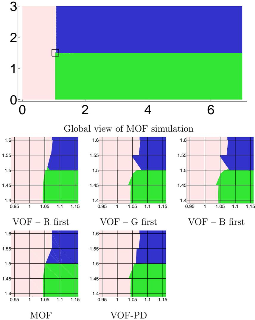
Fig. 5. Materials of triple point problem simulation, time  $T = 0.1$ . Eulerian runs (as Lagrangian step and remap to the initial orthogonal mesh) using different methods for material reconstruction are shown: global view on the entire computational domain for MOF method, and zooms to the three material junction for Young’s VOF method (with different material orderings), MOF, and Power Diagram based methods are shown.
