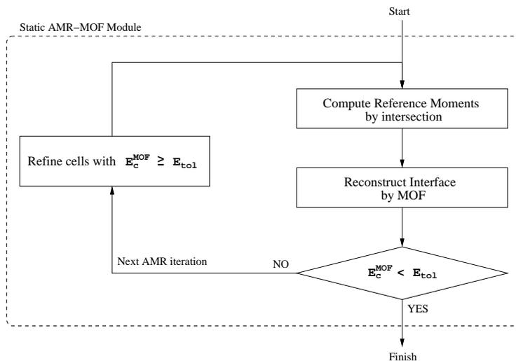
Figure 9: Flow-chart for static AMR-MOF interface reconstruction for initial representation of material configuration on AMR mesh.
