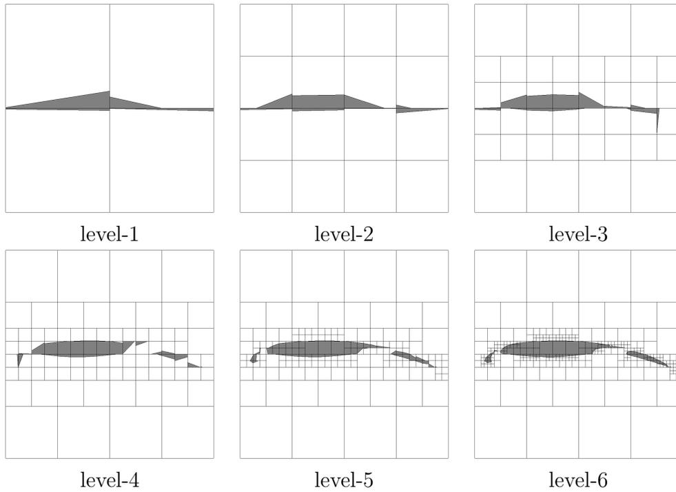
Figure 11: AMR-MOF interface reconstruction of multi-element airfoil configuration starting with one cell, i.e. the level-0 mesh is  $1 \times 1$  covering the domain of  $[0, 1]^2$ . Different levels of AMR-MOF reconstruction process are displayed.  $E_{tol} = 1.e-15$  is used as the refinement criterion.
