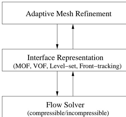
Figure 1: Conceptual structure of the adaptive mesh refinement strategy for interfacial flow computation. In volume-tracking methods (MOF or VOF), the *Interface Representation* module is typically composed of (i) interface reconstruction and (ii) advection steps.
