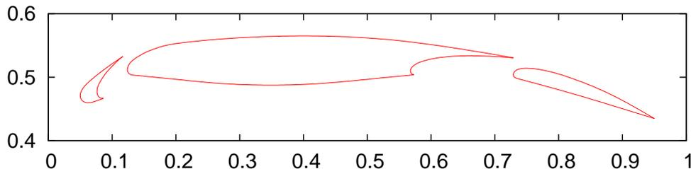
Figure 10: Multi-element airfoil configuration.
