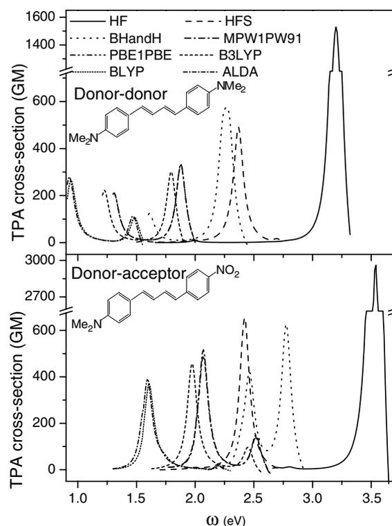
Fig. 1. Calculated TPA spectra of donor–donor (top panel) and donor–acceptor (bottom panel) molecules at different levels of theory (Table 1).
