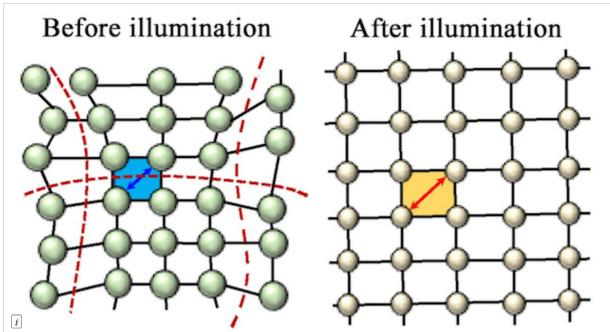
Constant illumination was found to relax the lattice of a perovskite-like material, making it more efficient at collecting sunlight and converting it to energy. The stable material was tested for solar cell use by scientists at Rice University and Los Alamos National Laboratory. Courtesy of the Light to Energy Team/Los Alamos National Laboratory
