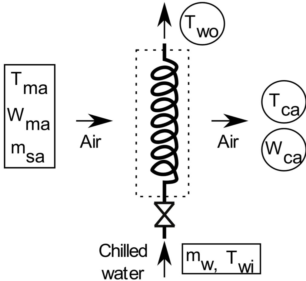
Model of cooling and dehumidification across a cooling coil:
