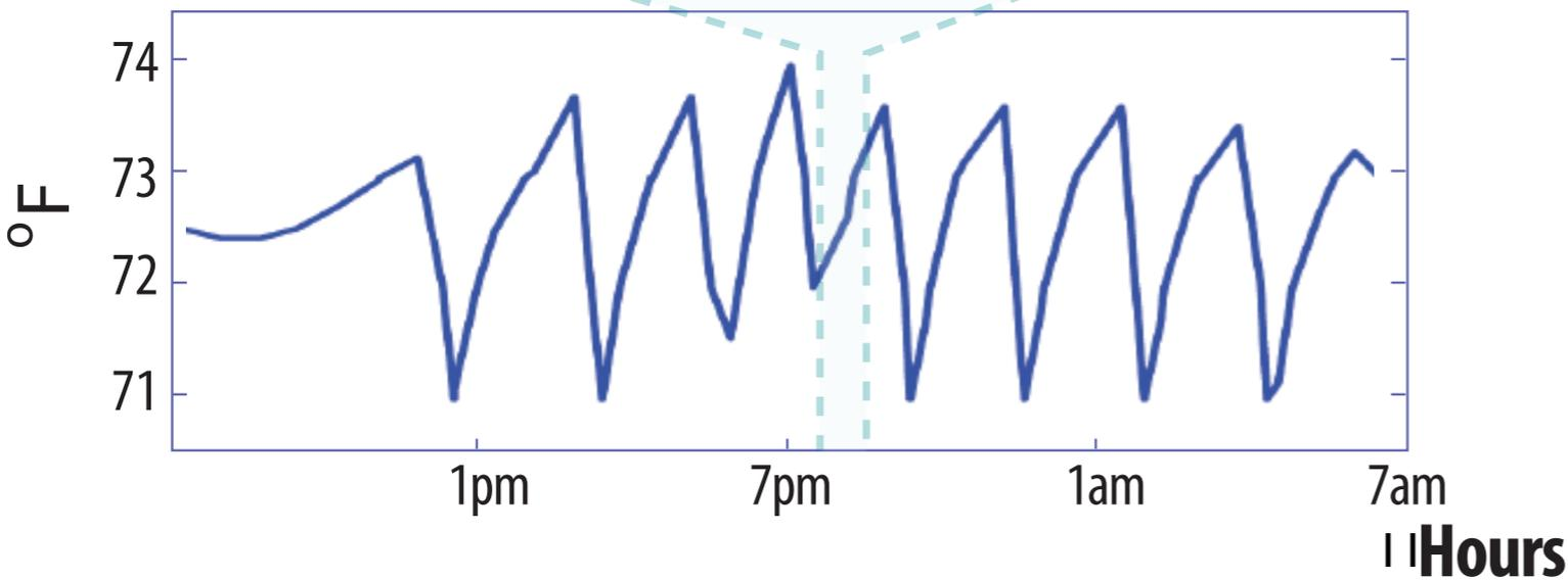
First experimental demonstration of a building providing "regulation" service\*
