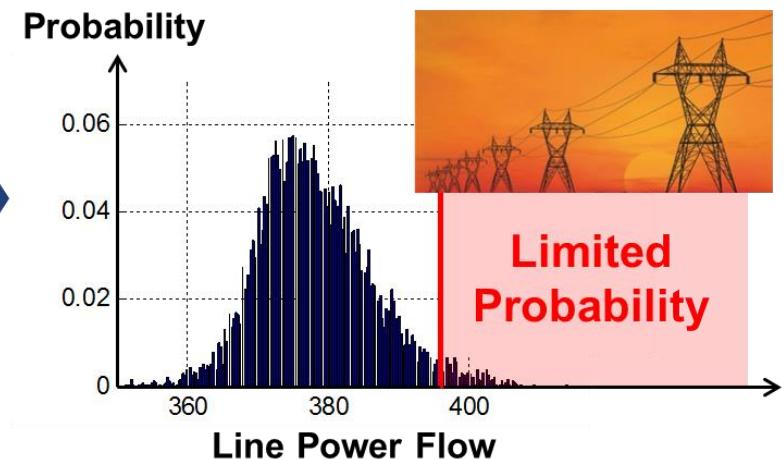
Chance-constrained **AC** Optimal Power Flow
