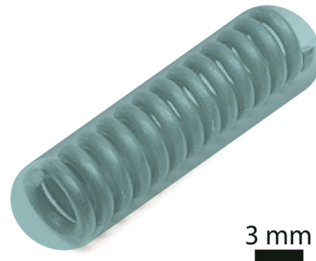
A mesoscale model; an elastic spring inserted in a flexible plastic tube (Weibel)
