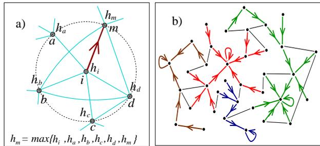
Figure 2: The gradient network. a) the gradient at node  $i$  is a directed edge pointing towards the largest increase of the scalar potential in the node’s neighborhood. b) an example of a gradient network.
