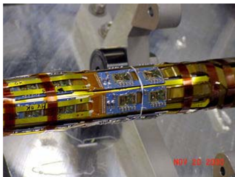
Electronics on beam pipe
