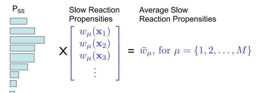
Use the fast sets' steady state probability distributions to scale the propensity functions of the slow reactions.
