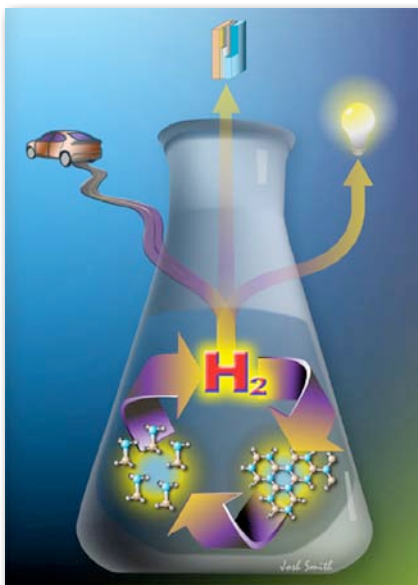
Figure 1. Artist's conception of the “one pot” regeneration of ammonia borane. Ammonia borane, on the left, releases hydrogen and is recycled back to polyborazylene on the right in a single vessel. Free hydrogen is available for a variety of applications. Design credit: Joshua Smith (Chemistry, C-DO)
