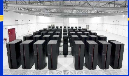
**IBM Supercomputer Jump** 32 processors 1.7 GHz and 128 Gbytes. 8.9 teraflops 5 terabyte memory
