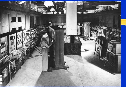
1945, **ENIAC** 30 tons, 19,000 vaccum tubes, 1,500 relays, and 200 kilowatts 350 flops, 400 bytes
