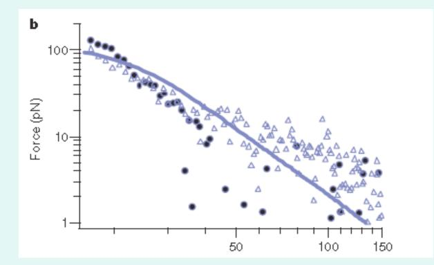
b,Measured repulsive force between a gold sphere and a silica plate in bromobenzene on a log–log scale (blue circles) and calculated force using Lifshitz's theory (solid line) including corrections for the measured surface roughness of the sphere and the plate. Blue triangles are force data for another gold sphere/silica plate pair.
