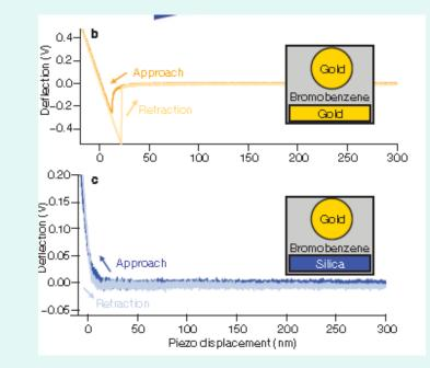
b, Deflection data showing attractive interactions between a gold sphere and a gold plate. c, For the case of the same gold sphere and a silica plate, deflection data show a repulsive interaction evident during both approach and retraction. Note that the deflection voltage signal is proportional to the bending of the cantilever.
