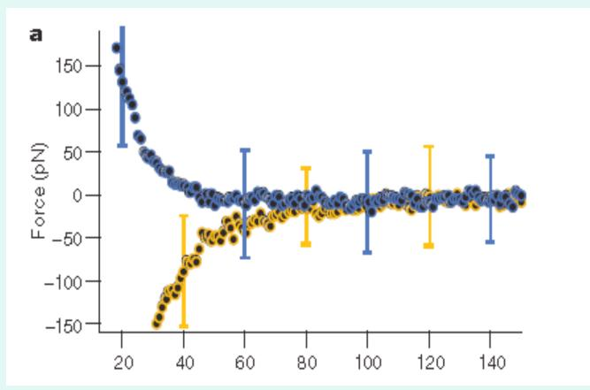
a, Blue (orange) circles represent the average of 50 data sets for the force between a gold sphere and a silica (gold) plate in bromobenzene.
