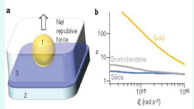
a, The interaction between material 1 and material 2 immersed in a fluid (material 3) is repulsive when  $\varepsilon_1(i\xi) > \varepsilon_2(i\xi) > \varepsilon_2(i\xi)$ . b, The optical properties of gold (1), bromobenzene (3) and Silica (2) are such that this inequality is satisfied. This leads to a repulsive force between the gold and silica surfaces.
