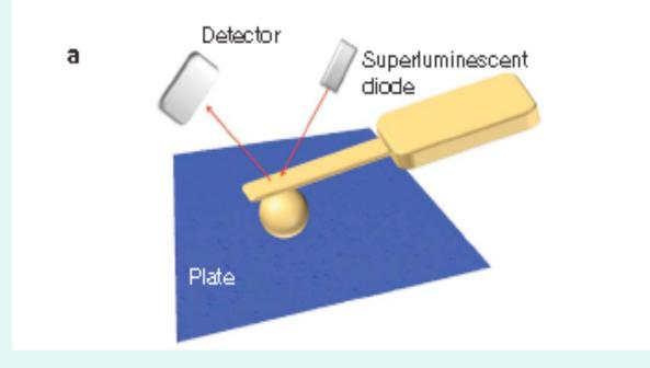
A sphere is attached to an atomic force cantilever, which is enclosed within a bromobenzene-filed cell for force measurements.
