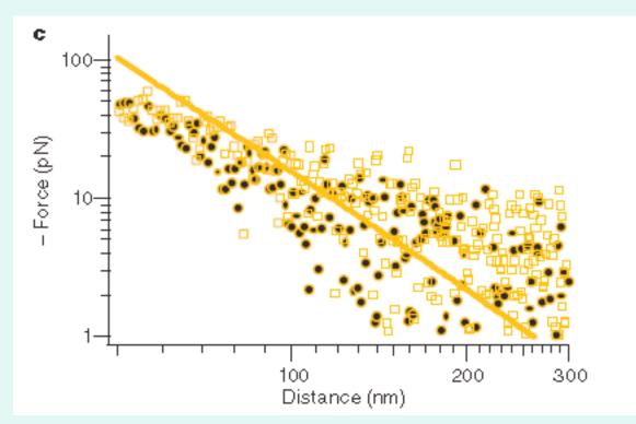
c, Measured attractive force on a log–log scale for two gold sphere/plate pairs (circles and squares) in bromobenzene. The calculated force includes surface roughness corrections corresponding to the data represented by the circles.
