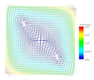
Figure 37: Analytical velocity field for shape-S case as described by Eq. (25). The velocity vectors are not scaled.  $32^2$  level-0 mesh is colored by the velocity magnitude.
