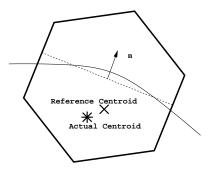
Figure 2: Stencil for MOF in two dimensions. The stencil for MOF interface reconstruction is composed of only the cell under consideration. The MOF method can be used for arbitrary polygonal cells (polyhedral cells in 3D). The solid curved line represents the true interface, and the dashed straight line represents the piece-wise linear, volume fraction matching interface at the cell.
