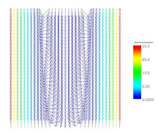
Figure 33: Analytical velocity field for droplet deformation problem as described by Eq. (24). The velocity vectors are not scaled.  $32^2$  level-0 mesh is colored by the velocity magnitude.
