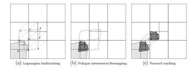
Figure 19: Moment advection on AMR mesh. Moment advection for child cells originated from the central parent cell is illustrated.
