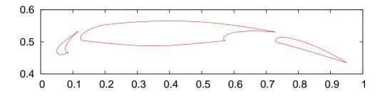
Figure 10: Multi-element airfoil configuration.
