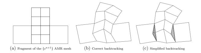
Figure 18: Lagrangian backtracking of the AMR mesh. Overlap area for simplified backtracking is shaded by horizontal lines, and gap is shaded by vertical lines.
