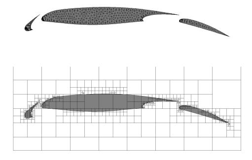
Figure 13: AMR-MOF interface reconstruction of stationary object. Threeelement airfoil geometry within  $1 \times 1$  mesh (level-0) covering the square domain  $[0, 1]^2$  is considered. Refinement is carried up to level-8, i.e. the maximum effective mesh resolution is  $256 \times 256$ . Top – original, bottom – AMR-MOF reconstruction.  $E_{tol} = 1.e$ -15 is used in the refinement criterion.
