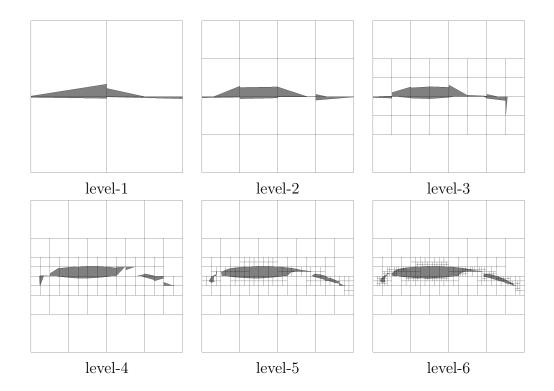
Figure 11: AMR-MOF interface reconstruction of multi-element airfoil configuration starting with one cell, i.e. the level-0 mesh is  $1 \times 1$  covering the domain of  $[0, 1]^2$ . Different levels of AMR-MOF reconstruction process are displayed.  $E_{tol} = 1.e$ -15 is used as the refinement criterion.
