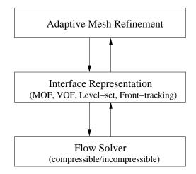
Figure 1: Conceptual structure of the adaptive mesh refinement strategy for interfacial flow computation. In volume-tracking methods (MOF or VOF), the *Interface Representation* module is typically composed of (i) interface reconstruction and (ii) advection steps.
