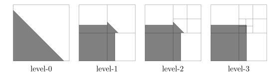
Figure 4: AMR-MOF interface reconstruction on adaptively refined meshes. From the left (level-0) to the right (level-3) refinement.
