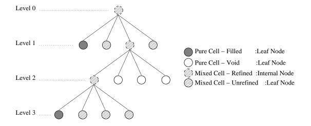
Figure 5: Quadtree structure of AMR-MOF reconstruction shown in Fig. 4. Correspondence between Fig. 4 established by introducing local enumeration of children of parent cell counter-clockwise starting from left-bottom child to left-top child. Then for each level left circle corresponds to left-bottom child and right circle correspond to left-top child.
