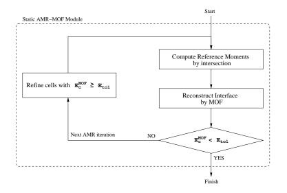
Figure 9: Flow-chart for static AMR-MOF interface reconstruction for initial representation of material configuration on AMR mesh.
