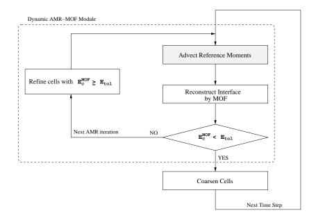
Figure 14: Flow-chart for dynamic AMR-MOF interface reconstruction and moment advection. The difference of the dynamic AMR-MOF module from the static AMR-MOF module, as shown in Fig. 9, is reference moment computation step. For dynamic case, the reference moment is computed by advection step, as indicated with gray box.
