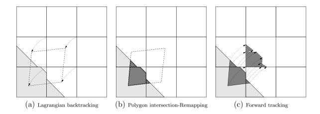
Figure 17: Moment advection by Lagrange+remap strategy. The moment advection process for the central cell-c on  $3 \times 3$  local stencil is illustrated.
