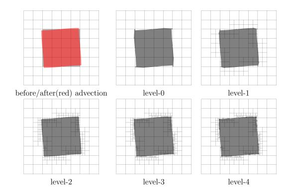
Figure 15: One time step of the advection  $(\Delta t = \frac{1}{32})$  of a square box using nonlinear velocity field with T = 8.0 as described in Eq. (7). Initial square box configuration is defined by  $[0.25, 0.75]^2$ . Level-0 mesh is  $8 \times 8$  covering the square domain  $[0, 1]^2$ . Left-top figure shows exact material configuration before (gray) and after (red) the advection. The others are after one step of the advection using different levels of AMR.  $E_{tol} = 1.e$ -15 is used.
